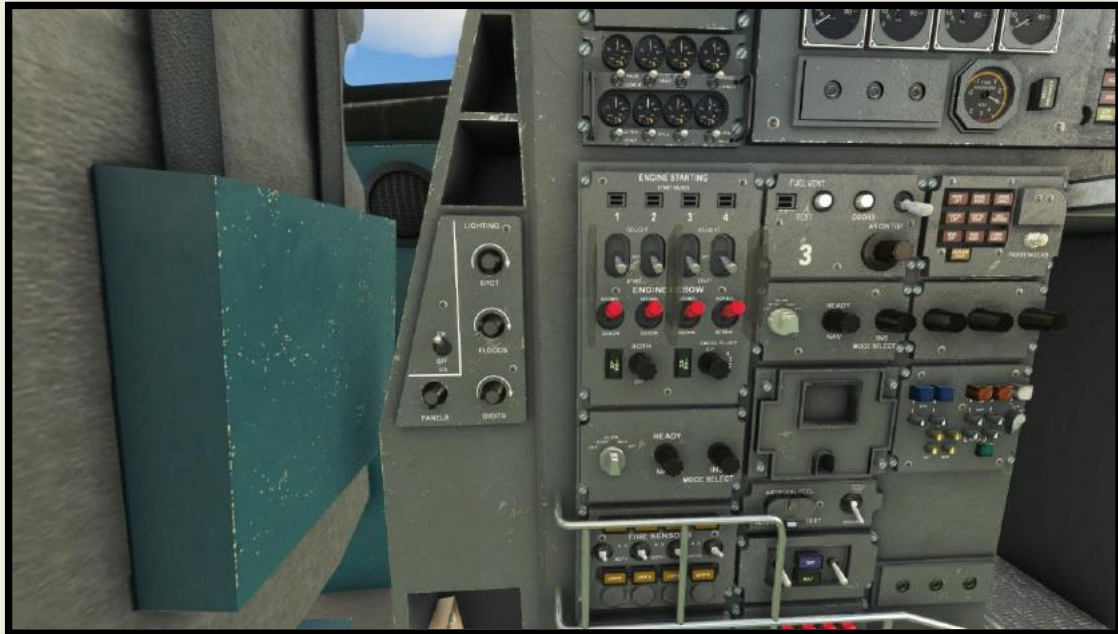
Engine Start switches are labelled, centre of image, 1-2-3-4
