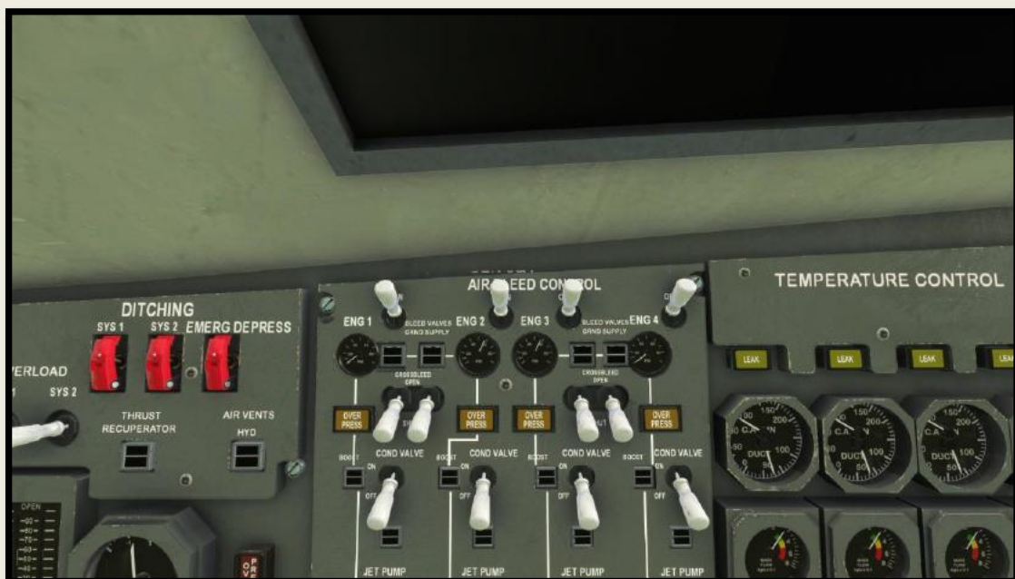
Air Bleed Control switches ( OPEN POSITION, top centre )
